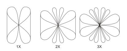
Figure 4-17. Long Wire Radiation Patterns.
