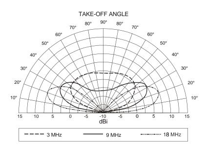
Figure 4-15. Inverted Vee (Vertical Pattern).
