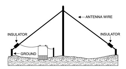
Figure 4-30. Vertical Half-Rhombic Antenna.
