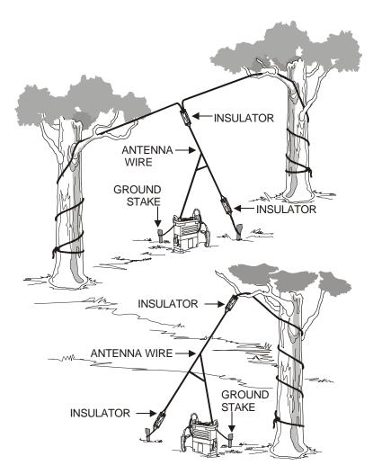
Figure 6-9. Improvised Vertical Half-Wave Antenna.
