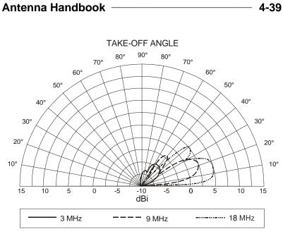
Figure 4-31. 50-Foot Vertical Half-Rhombic (Vertical Pattern), 500 Feet Long.
