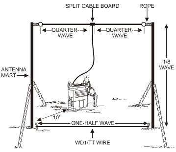
Figure 6-12. Yagi Antenna.
