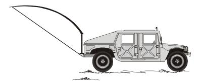
Figure 4-34. AN/MRC-138 with NVIS Antenna.
