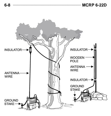
Figure 6-4. Field Substitutes for Support of Vertical Wire Atennas.
