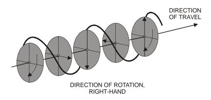
Figure 2-5. Circular Polarization.
