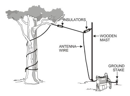
Figure 6-5. End-Fed Half-Wave Antenna.
