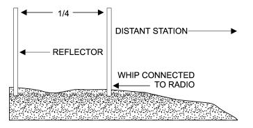
Figure 4-6. Vertical Whip with Reflector.
