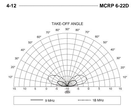
Figure 4-7. 10-Foot Vertical Whip (Vertical Pattern).
