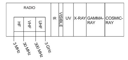
Figure 1-1. Electromagnetic Spectrum.
