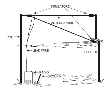
Figure 4-22. Sloping Vee Antenna.
