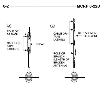
Figure 6-1. Emergency Repair of Broken Whip.
