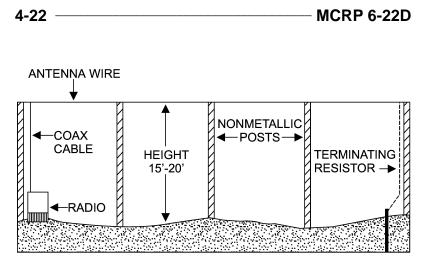
Figure 4-16. Long Wire Antenna.
