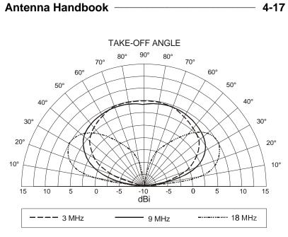
Figure 4-11. 8-Meter Half-Wave Dipole (Vertical Pattern).
