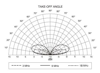
Figure 4-3. 32-Foot Vertical Whip, Vertical Pattern.
