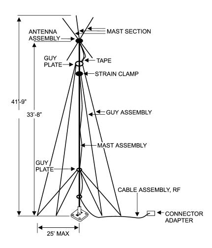
Figure 5-1. Installed OE-254 Antenna.
