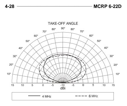
Figure 4-21. 40-Foot Inverted L (Vertical Pattern), 100 Feet Long.
