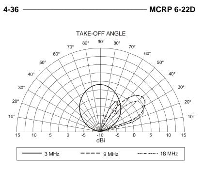
Figure 4-28. 250-Foot Sloping Wire (Vertical Pattern).
