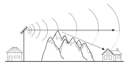
Figure 1-7. Diffracted Wave.
