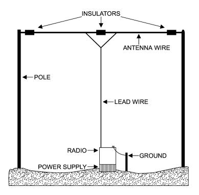
Figure 4-10. Half-Wave Dipole Antenna.
