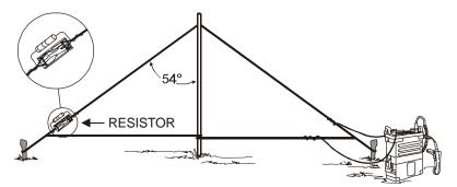
Figure 6-10. Vertical Half-Rhombic Antenna.
