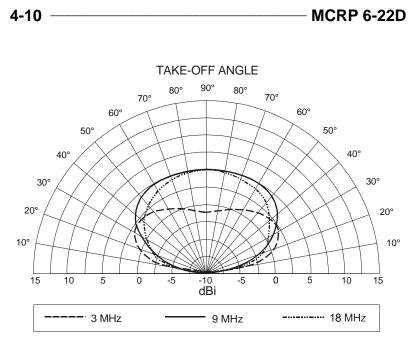
Figure 4-5. AS-2259 Vertical Radiation Pattern.
