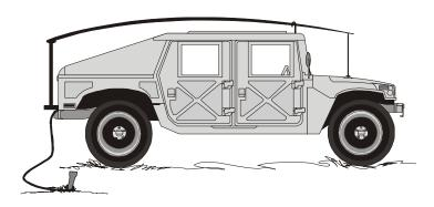
Figure 4-35. AN/MRC-138 with Stationary NVIS Antenna.
