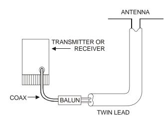
Figure 3-3. Balun Placed at the Transmitter or Receiver.
