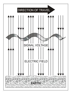
Figure 2-3. Vertical Polarization.
