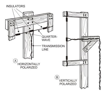
Figure 6-7. Center-Fed Half-Wave Antenna.
