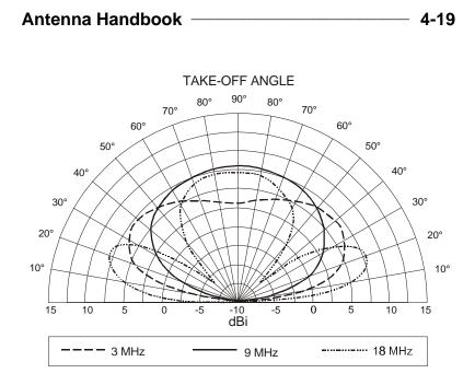
Figure 4-13. 12-Meter Half-Wave Dipole (Vertical Pattern).
