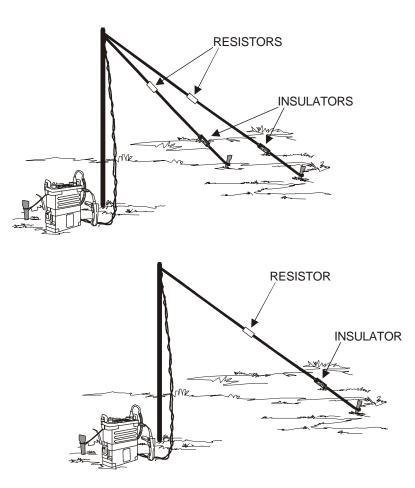
Figure 6-14. Sloping Vee Antenna.
