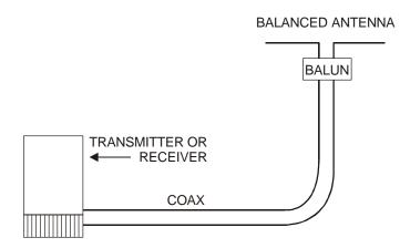
Figure 3-2. A Balun Placed at the Antenna.
