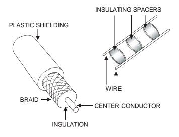
Figure 4-1. Antenna Feed Lines.
