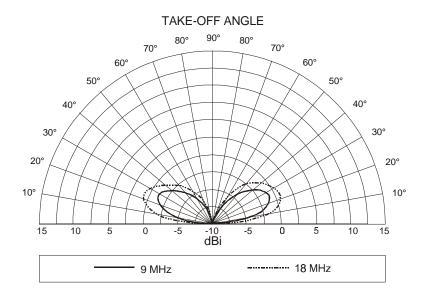
Figure 4-8. 15-Foot Vertical Whip (Vertical Pattern).
