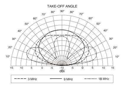
Figure 4-12. 10-Meter Half-Wave Dipole (Vertical Pattern).
