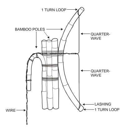
Figure 6-8. Bent Bamboo Antenna.
