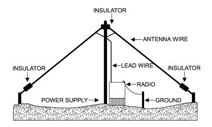
Figure 4-14. Inverted Vee Antenna.
