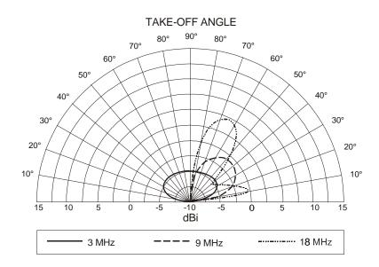
Figure 4-27. 100-Foot Sloping Wire (Vertical Pattern).
