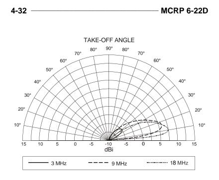
Figure 4-24. 40-Foot Sloping Vee Antenna (Vertical Pattern), 500 Feet Long, 45° Apex Angle.
