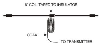
Figure 4-2. Coax RF Current Choke.
