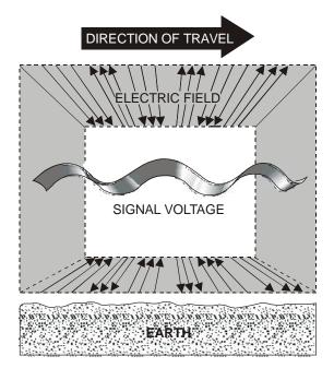
Figure 2-4. Horizontal Polarization.
