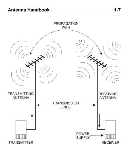
Figure 1-3. Typical Radio Link.
