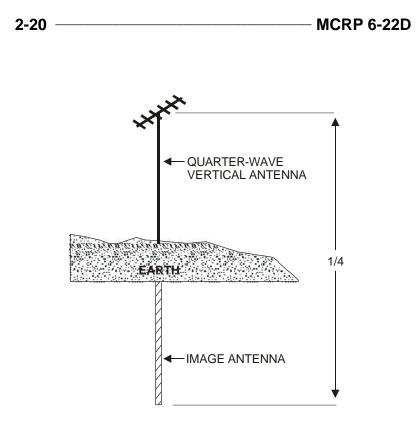
Figure 2-9. Quarter-Wave Antenna Connected to Ground.
