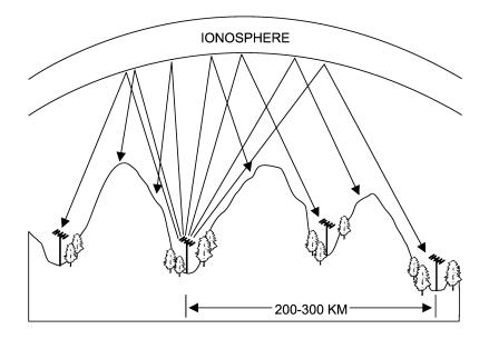
Figure 4-33. NVIS Propagation.
