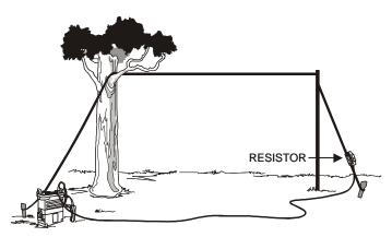
Figure 6-11. Long Wire Antenna.
