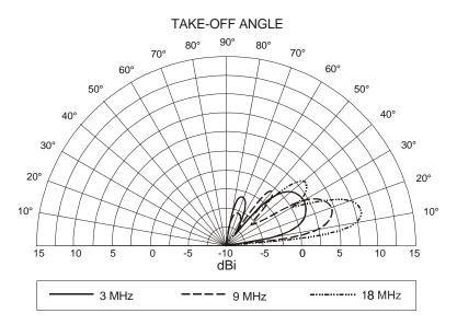
Figure 4-29. 234-Foot Sloping Wire (Vertical Pattern).
