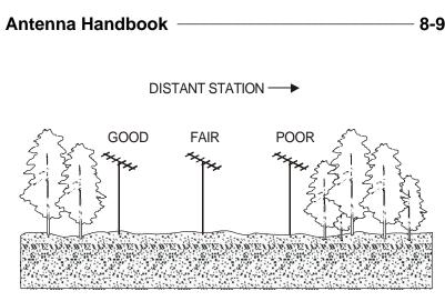
Figure 8-4. Directional Antennas Sited in a Clearing.
